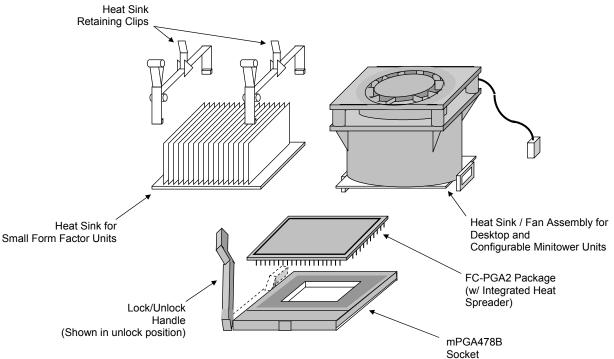
Figure 2–10. Processor Assembly And Mounting
